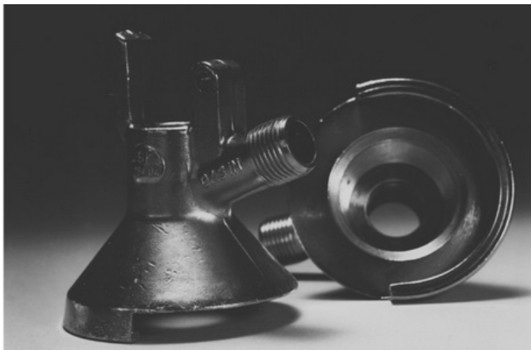
Figure 5 - Gas valve for draft beer produced in hot pressed brass and plated with a tin/nickel alloy (Photo provided by Micro Matic A/S Denmark).
